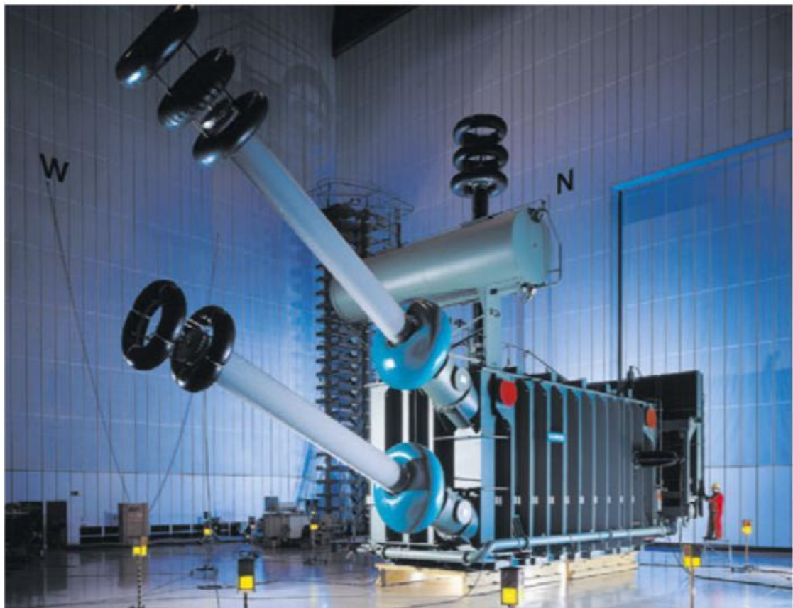
Converter transformer for HVDC bipolar transmission system \pm 500\text{kVdc} ; 2,500MW: single-phase; 420kVac; 515kVdc; 397MVA; wye system (on left) and delta system (on right).
