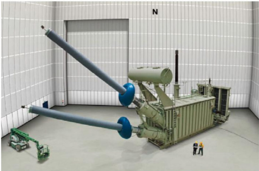
Converter transformer for HVDC bipolar transmission system \pm 800\text{kVdc} , 6,400MW; 2,071km: single-phase; 550kVac, 816kVdc; 321MVA; high pulse wye system feeding.
