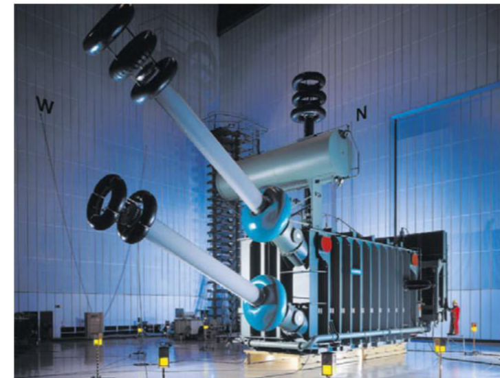
Converter transformer for HVDC bipolar transmission system \pm 500\text{kVdc} ; 2,500MW: single-phase; 420kVac; 515kVdc; 397MVA; wye system (on left) and delta system (on right).
